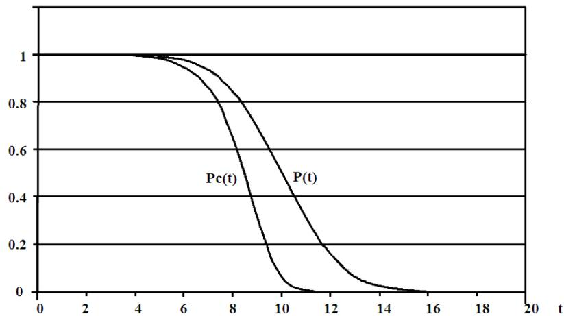
**Figure 11** The reliability functions by the normal distribution of time to failure and the sinusoidal load rate
