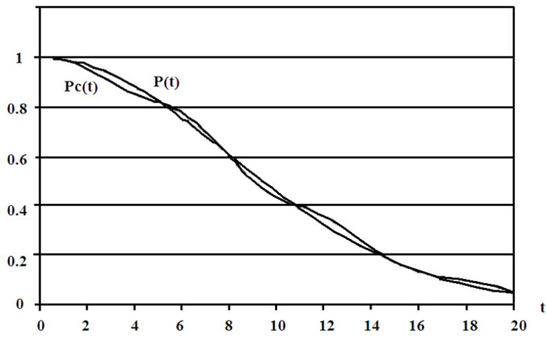
**Figure 9** The reliability functions by the Rayleigh distribution of time to failure and the sinusoidal load rate
