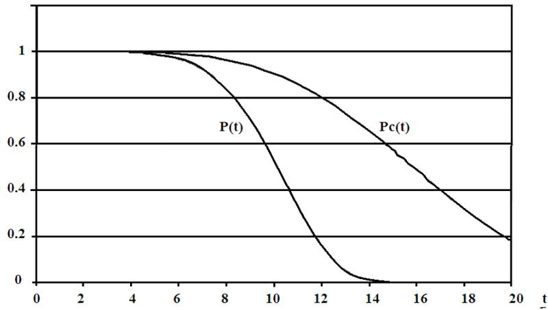
**Figure 8** The reliability functions by the Weibull distribution of time to failure and the non-linear load rate
