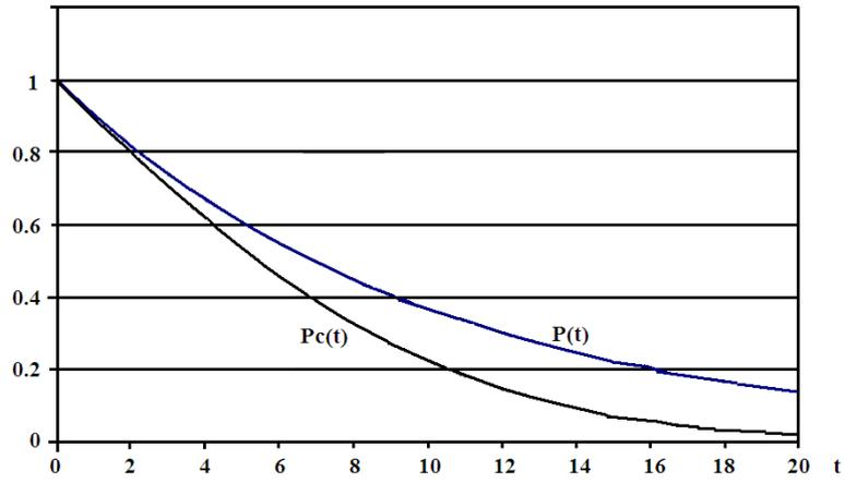
**Figure 4** The reliability functions by the exponential distribution of time to failure and the linear load rate
