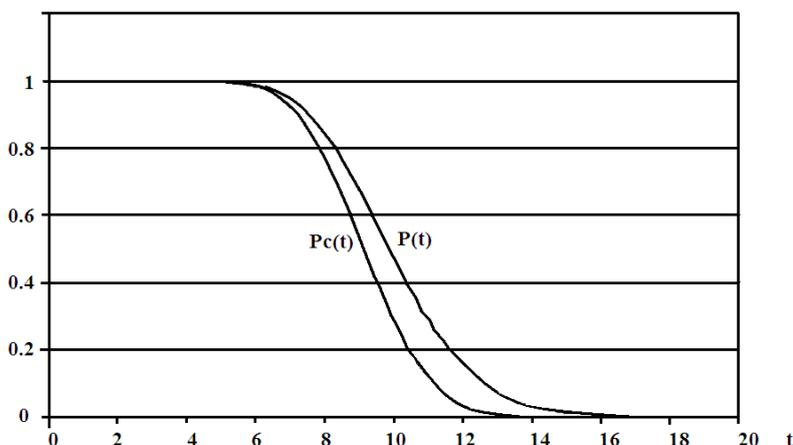
**Figure 6** The reliability functions by the gamma distribution of time to failure and the linear load rate
