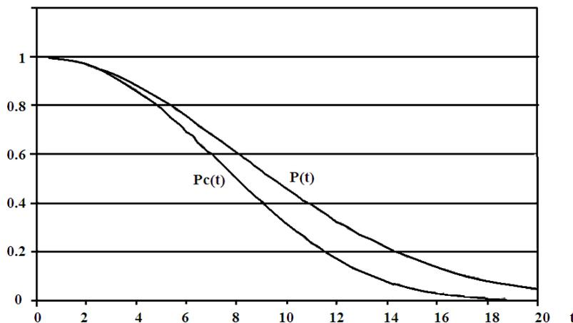
**Figure 7** The reliability functions by the Rayleigh distribution of time to failure and the linear load rate
