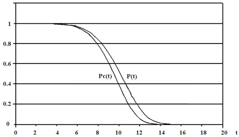
**Figure 5** The reliability functions by the Weibull distribution of time to failure and the linear load rate
